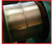
9) Repeat the process of applying a retaining compound to the shaft area for the second and outer repair sleeve. Again, use the sleeve driver to gently tap the second sleeve into place, (right image). Detach and peel away the drive ring from the sleeve and wipe away excess retaining compound. Sleeves must be allowed to sit for approximately one hour so the retaining compound has time to lock the sleeves into place.
