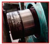
8) The drive ring attached to the sleeve is perforated and must be peeled away once the sleeve is in place.
