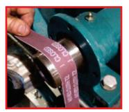
5) With drum shaft now exposed, inspect closely for pitting or grooves caused by neglect from not applying grease. Clean the end of the shaft with solvent to remove all old grease. If drum shaft is pitted, use emery cloth, (right image), and remove rust until drum shaft is smooth.
