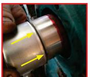
7) Apply some industrial retaining compound to the shaft in order for first sleeve is to be installed, (right image).
