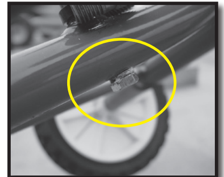
Guncart drain location on RG25
